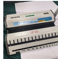
Rosback 240B Vacuum Feed Slit/Score/Perforation Machine $14,995 $9,995 Slit, score & perf substrates up to 14pt card; sizes from 7.5" x 7.5" up to 30" x 30"; up to 25k ft/hr
