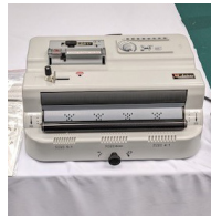
Rosback 240B Vacuum Feed Slit/Score/Perforation Machine $14,995 $9,995 Slit, score & perf substrates up to 14pt card; sizes from 7.5" x 7.5" up to 30" x 30"; up to 25k ft/hr
