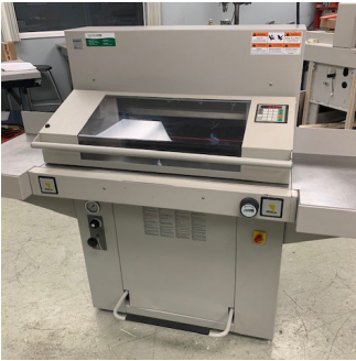
EBA 550EP Paper Cutter $8,495 $7,995 Hydraulic cut&clamp; 21.6" cut width; incl. side tables
